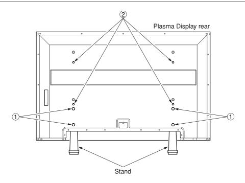
1 Turn the plasma display over and place it screen-first onto a table which has a soft cloth draped over it.
